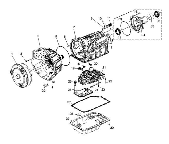
To correct this condition the control valve body spacer plate (305) must be replaced. The electrical connector seals (9, 10), fluid pump seals (18, 19), center support seal (20) and the filter plate assembly (311) should also be replaced. These parts are included in the filter plate kit listed below.
