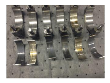
If the main and/or rod bearings are found to be the cause of the debris, before deciding whether to replace the engine or repair it, refer to the Service Procedure below before making that determination.
