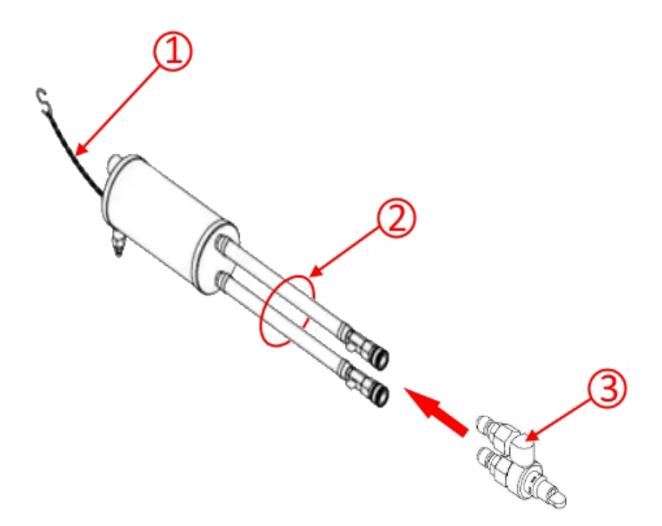
1. Attach *GE-52079* Tool, Coolant System Fill lines (2) to *GE-52079-10* Adapter, Coolant System Fill Tool (3).
