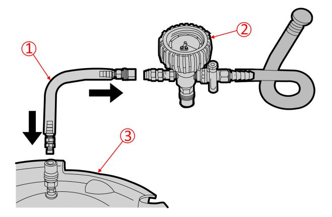
1. Attach the vacuum hose (1) to the vacuum gauge assembly (2) and the vacuum tank (3).
