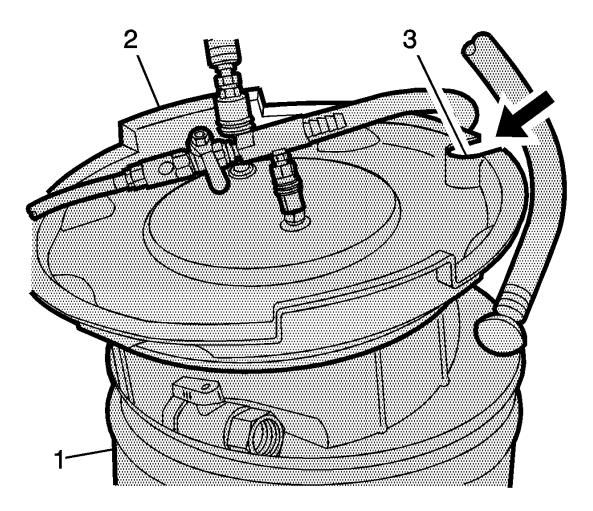
**Note:** Use a 50/50 mixture of DEX-COOL antifreeze and clean, drinkable water. Always use more coolant than necessary. This will eliminate air from being drawn into the cooling system.
