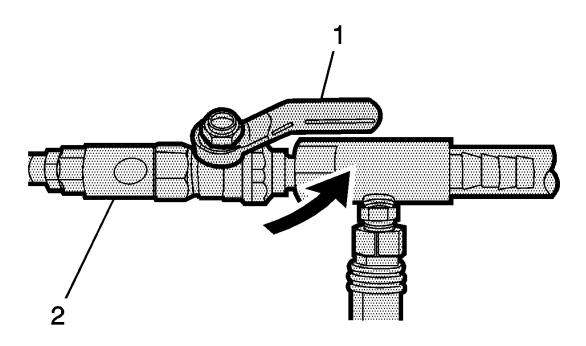
1. Open the valve (1) on the venturi assembly (2).
