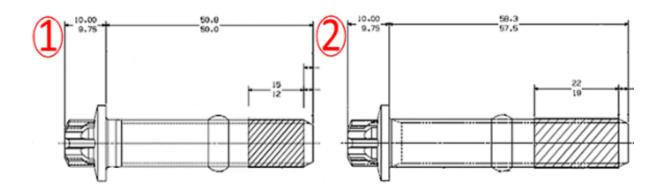
Service stock half shafts may include POA retainer assemblies that have the shorter bolt (1), these assemblies may require to be exchanged with new retainer assemblies that have the longer bolts (2).
