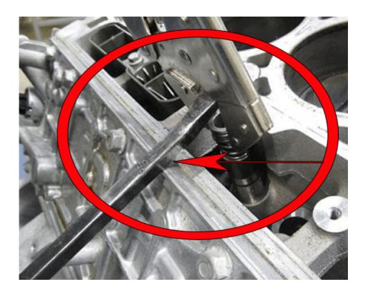
**Note:** Be sure *NOT* to pry on the sealing surface of the block, as shown in the illustration above.
