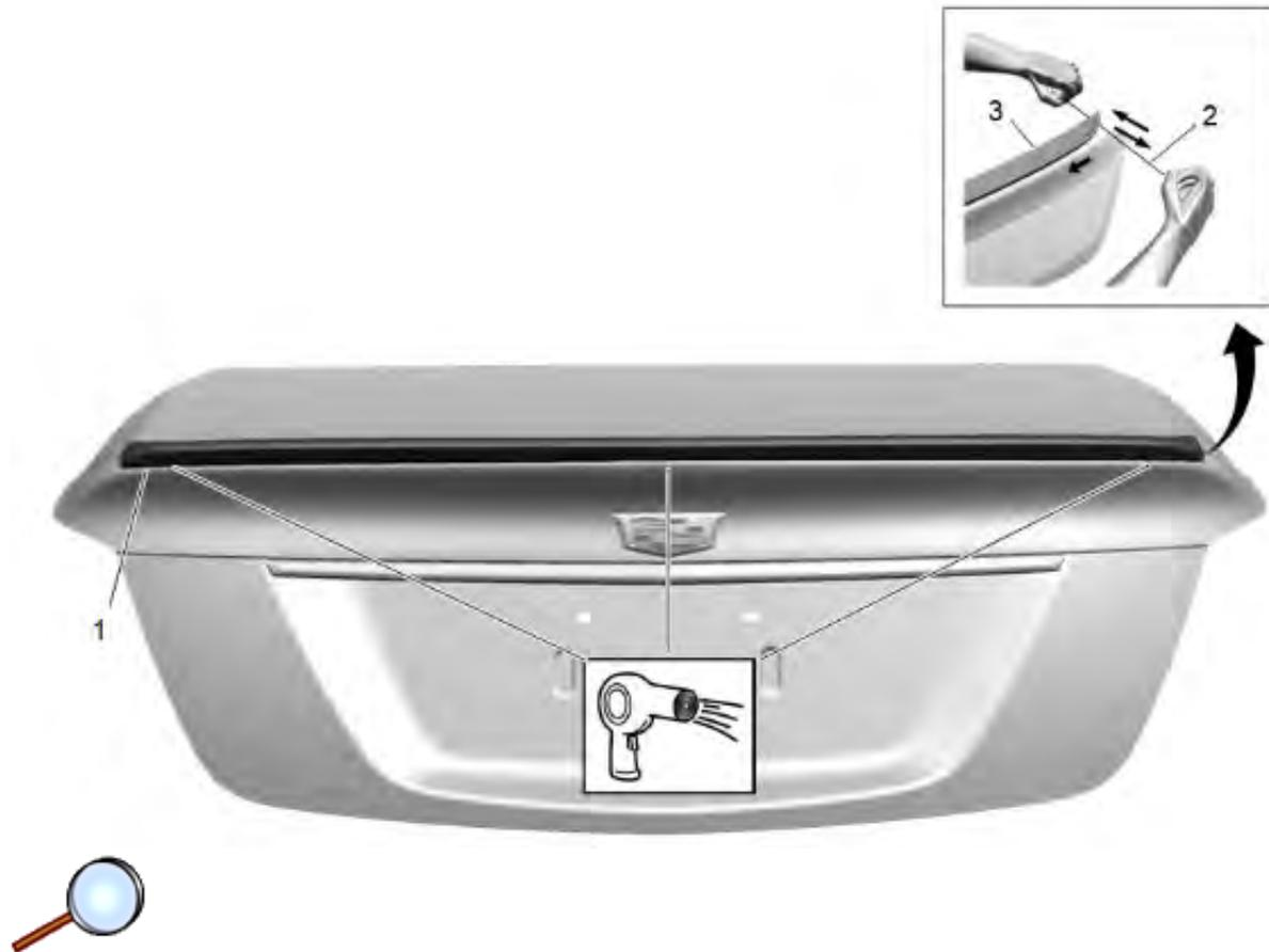
Note: If vehicle is not equipped with production spoiler, continue to Drilling Instructions section.
