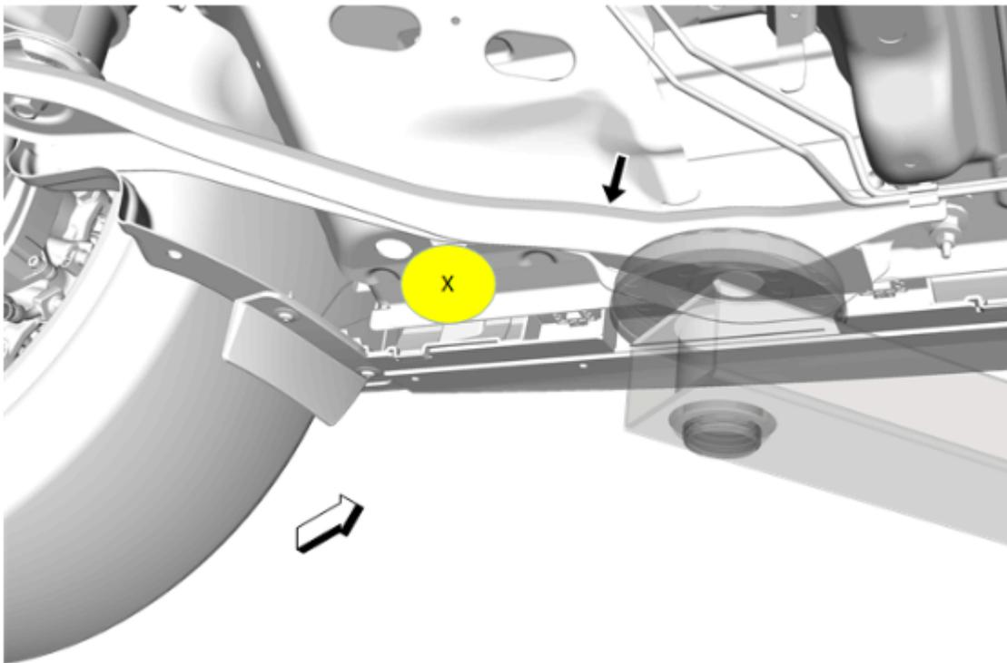
When lifting the vehicle with a frame-contact lift, cover the inner and outer edges of the rear suspension bracket (arrow). Use the cutout in the rocker molding to correctly position the pad
