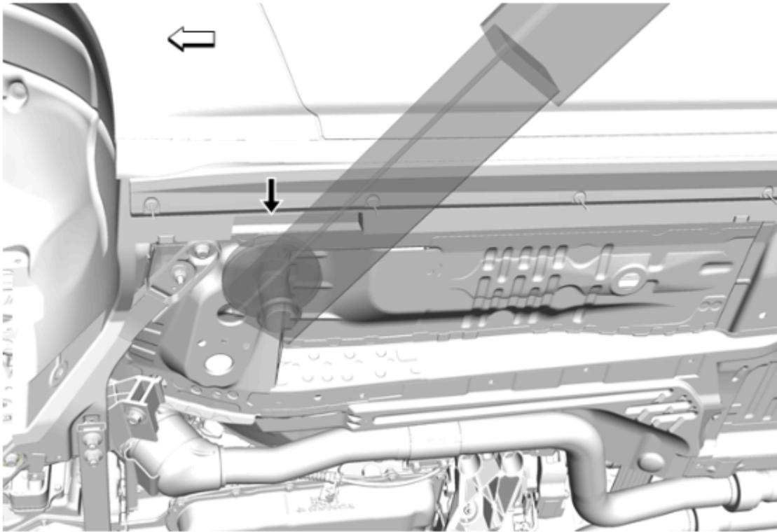
When lifting the vehicle with a frame-contact lift, position the pad as close as possible to the rocker molding cutout.
